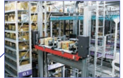
High-throughput mini load AS/RS Stores different-sized cardboard boxes and facilitates case shipping
