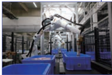
Piece-picking robot Carefully and gently picks individual items of various sizes and weights
