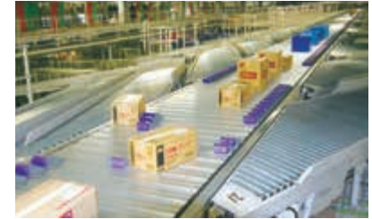
High-speed sorter - Surfing Sorter
