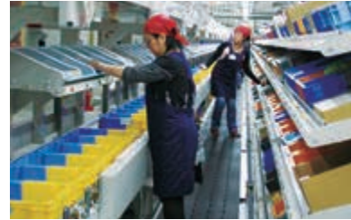
Pick-to-light system - Digital Pick System
