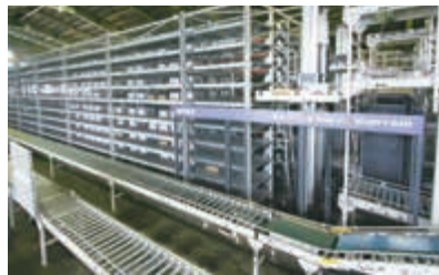
High-throughput multi shuttle mini load AS/RS - Shuttle Rack-M
