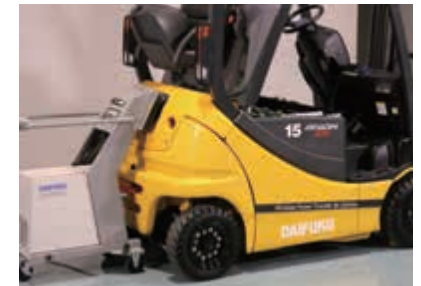
(Picture 2) Wireless battery charging system for electric forklifts – D-PAD
