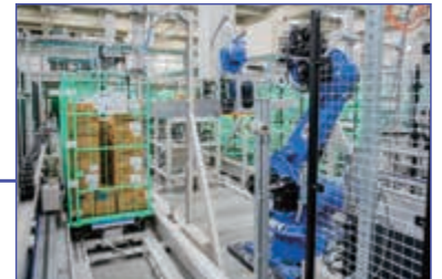
Case-palletizing robot Rapidly palletizes cases of various shapes and sizes
